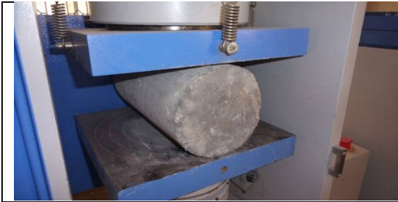
Figure 7 – Testing of Cylinder specimens
