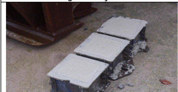
Figure 5 – Casting of Cube specimens
